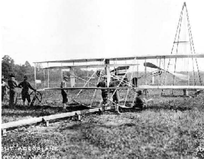
The Wright Military Flyer is set up on a launching rail at College Park in 1909.
