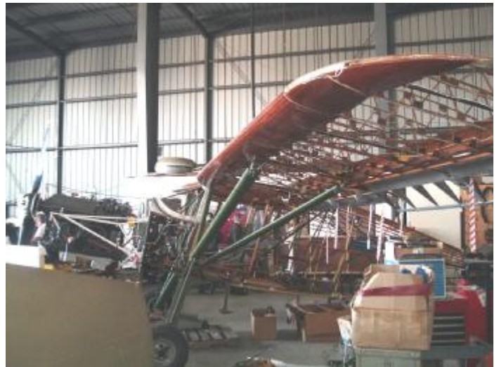
© Photo by Dave Flood Note the wood structure in wing and fuselage – to be fabric covered.
