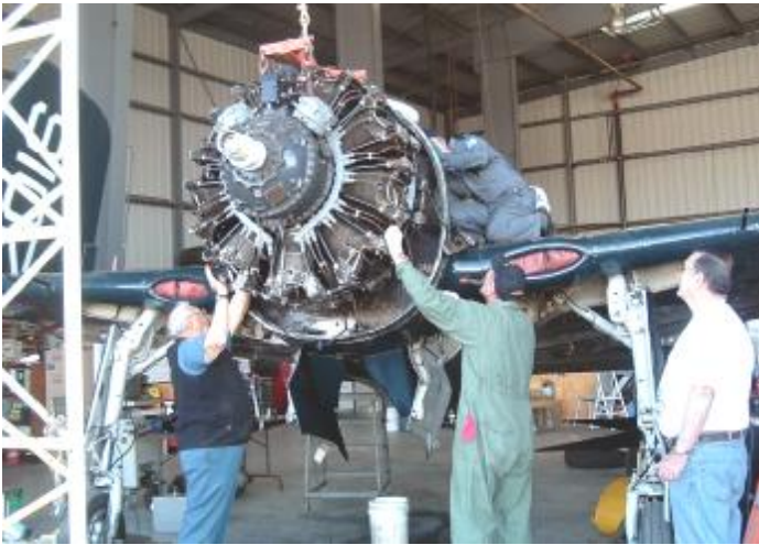
© Photo by Dave Flood Easing the R2800 off the Bearcat's mounts. From the left: Joe Peppito, Chris Rushing and Ken Barger. Ken Kramer, the Crew Chief, is on the wing.
