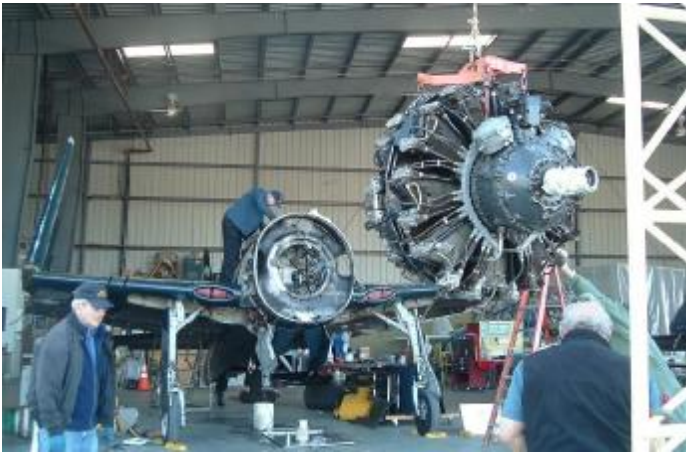
© Photo by Dave Flood The engine is out for repairs to the blower section. On the left is Dean Browne. Gary Barber is on the wing.
