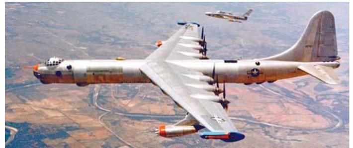
Convair JRB-36F Peacemaker, with "six turnin' and four burnin'". Note the special extensions on the wing tips to accommodate two RF-84 jets as "piggy-backs."
