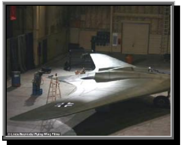
A full scale replica of the Ho 229 bomber made with materials available in the 1940s.
