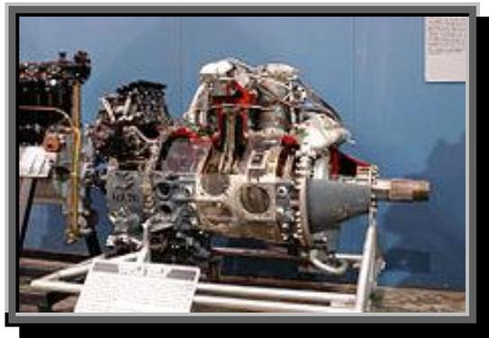
✈️ A Wright R-3350 radial engine, showing, R to L, propeller shaft, reduction gearcase, magneto (silver) with wiring, two cylinders (rear with connecting rod), impellor casing (and induction pipe outlets) and injection carburetor (black); separate accessory gearbox at extreme left
