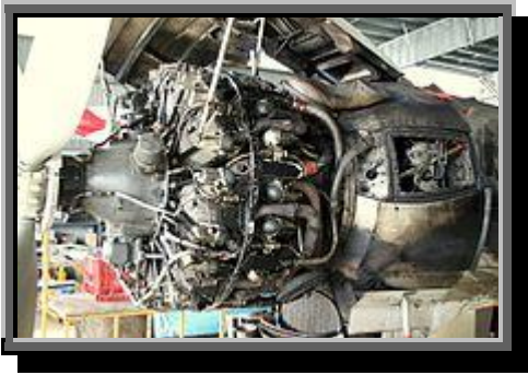
✂ Wright R-3350 Turbo-Compound radial engine fitted at the Number Four position on the starboard wing of a Lockheed Super Constellation
