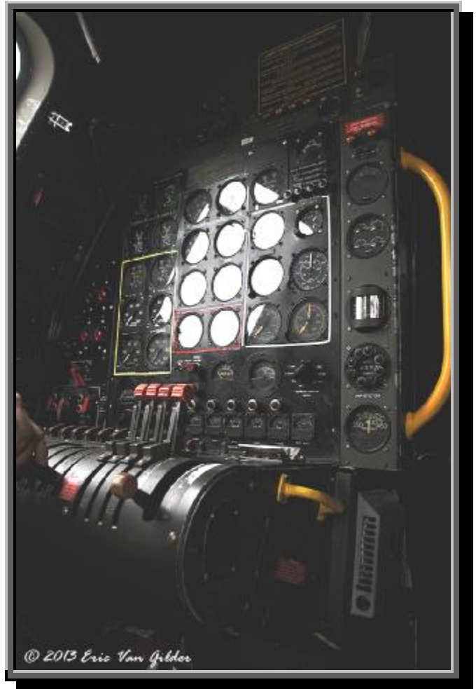
Here's the flight engineer's panel, located behind the co-pilot's seat. The flight engineer starts and controls the engine power settings and synchronizes the engines during takeoff and cruise. He also manages the various aircraft systems. Note the throttle, mixture, and propeller pitch control levers, which duplicate those available to the pilots.
