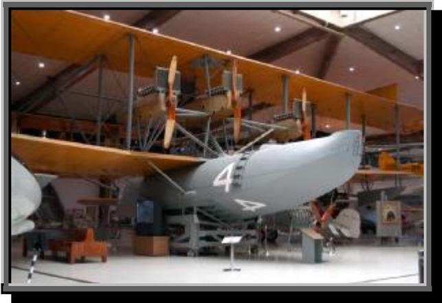
When completed, a mammoth wooden hull constructed of two levels of cedar planking supported sweeping wings that stretched to 126 feet. Four Liberty V-12 engines (three "pullers" and one "pusher") fed from tanks containing 1,891 gallons of gasoline provided 1,600 horsepower, enabling a top speed of 85 miles per hour when the aircraft was at its fully loaded weight of 28,000 lb.
