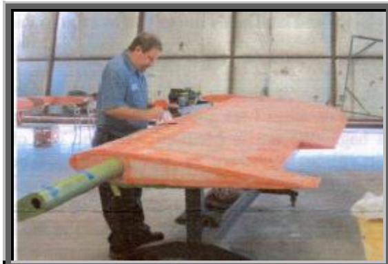
PBY Catalina elevator with fabric expertly applied.
