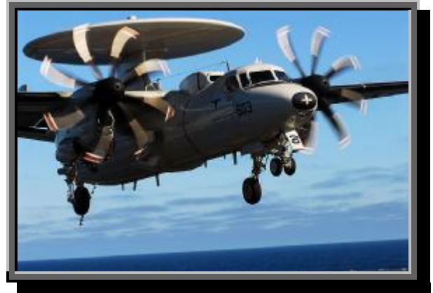
E-2C Hawkeye of VAW-117 landing aboard USS John Stennis (CVN74) in the Pacific. Note 8-bladed "scimitar" propellers.
