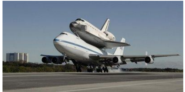
© NASA Photo NASA 747-100 (SCA) landing with a shuttle aboard. Note the "nose-up" approach. Easy does it !
