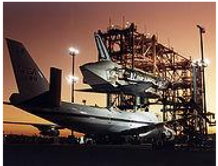
© NASA Photo The shuttle being lifted off the 747 (SCA) by the Mate-Demate Device – at the end of the journey at the Kennedy Space Center in Florida.
