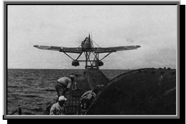
The "Glen" was launched via catapult from a I-25 class Japanese submarine.
