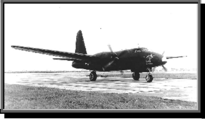
Taxiing tests demonstrated that the Lockheed P2V-1's landing gear might fold while bearing the Turtle's extreme weight before carrying it airborne. And during taxi turns its landing gear struts could fail carrying such a load. For that reason, the Turtle was only partially filled with fuel before it was positioned at the head of Perth, Australia's Pearce Aerodrome runway 27 in at 7 A.M. on September 29th, 1946.
