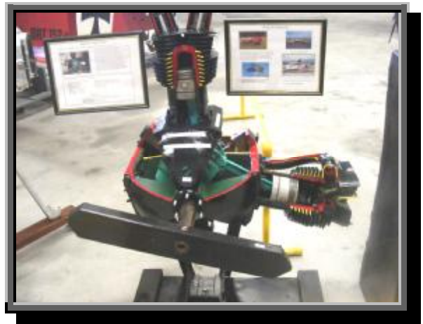
Cut-Away Model of a Kinner B-5 radial engine which was renovated, painted and set on a pedestal, with attached descriptive sheets. It is now on display in our Aviation Museum, thanks to the Radial Engine Class.
