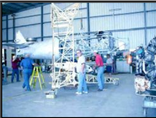
The crew fitting the spar to the fuselage.
