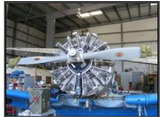
The engine and the propeller have been installed, and the crew is ready to work on the wiring, instrumentation and controls.
