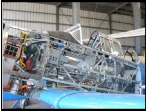
Much of the cockpits, wiring and cables have been installed.
