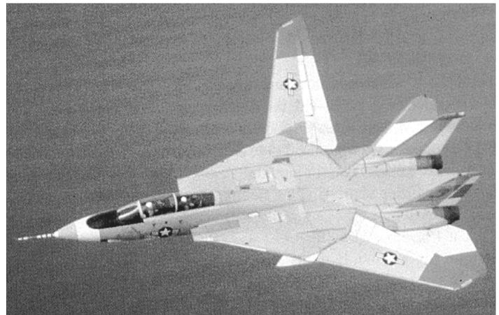
**F-14 in flight with left wing fully swept and right wing fully extended. Note control surface position on left wing required to hold the aircraft level.** NASA photo
