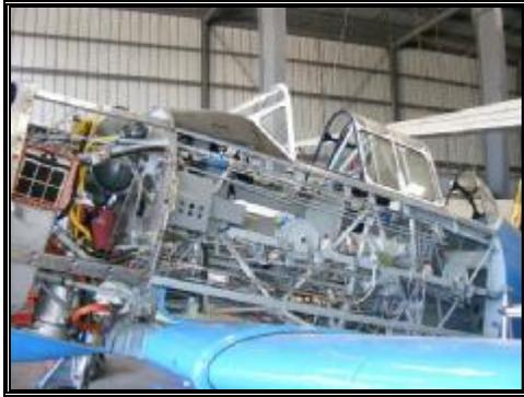
Much of the cockpits, wiring and cables have been installed.
