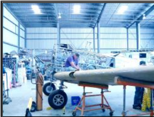
Tom Branch tightening bolts on the wing. Note the gear has been attached.
