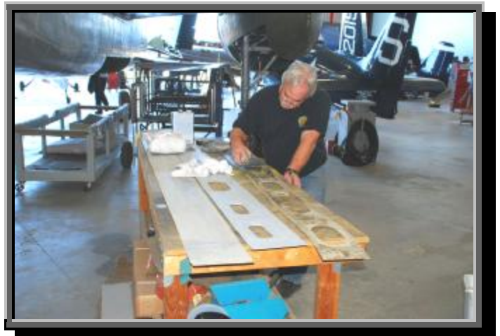
© Photo by Dan Newcomb Col. Dave Neel working on a PBJ wing close-out panel.
