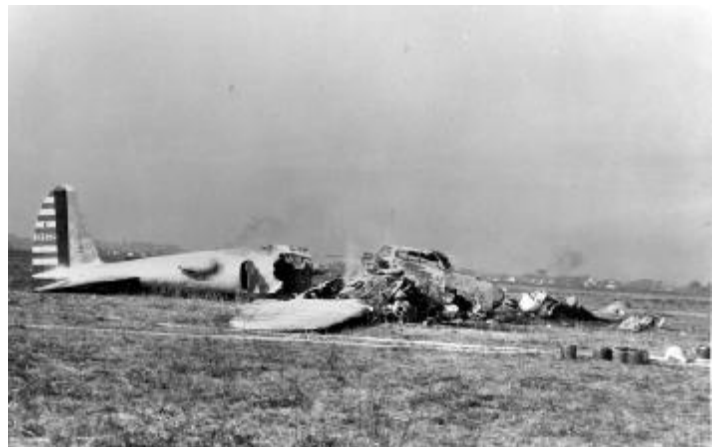
The Boeing Model 299 after the crash. It's ironic that the rudder and elevators that had not been unlocked are still intact after the crash.
