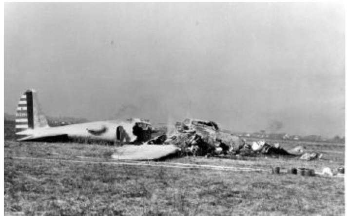
**The Boeing Model 299 after the crash. It's ironic that the rudder and elevators that had not been unlocked are still intact after the crash.**
