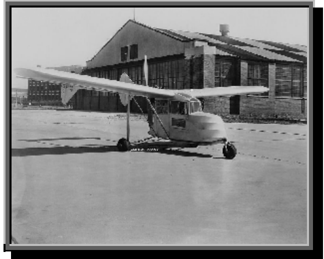
The Fred Weick-designed W-1. Note tricycle landing gear; twin rudders and pusher prop.
