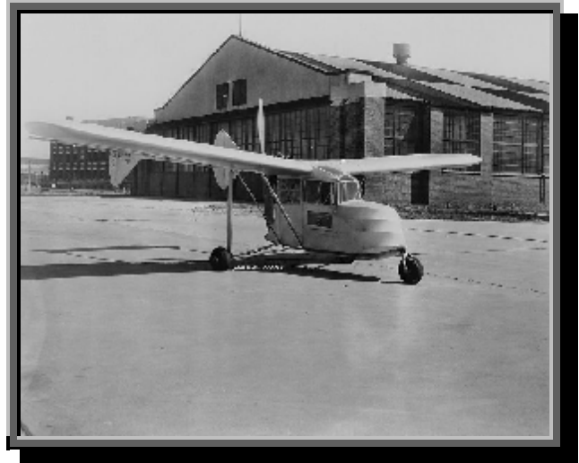
The Fred Weick-designed W-1. Note tricycle landing gear; twin rudders and pusher prop.
