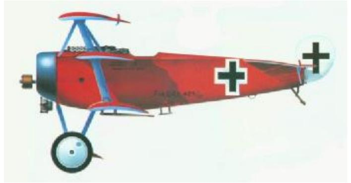
Here is one of the planes that the Red Baron flew and in which he scored many of his victories. It is the Fokker Dr. I Triplane, Built in 1917, powered by a Thulin-built Le Rhone 9J 9-cylinder air-cooled rotary 110 HP engine. It weighed 1,289 pounds, had a maximum speed of 103 mph, and a ceiling of 19,685 feet. Its armament was two synchronized Spandau machine guns.
