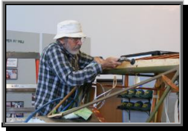
© Photo by Dave Flood Barry Roberts doing his custom work on our Fairchild F-24. Barry is remaking both doors on the F-24, and doing a wonderful job. Thanks, Barry !
