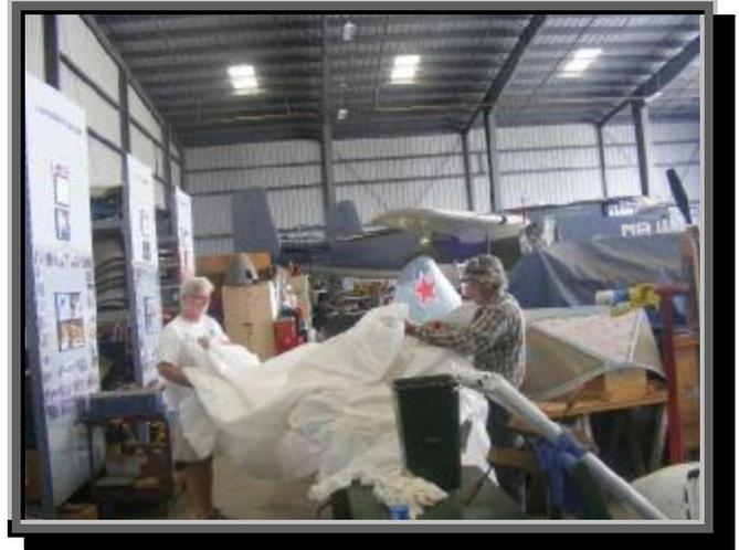
George and Barry unboxing the fiber covering prior to slipping it on the fuselage, from tail to cockpit.
