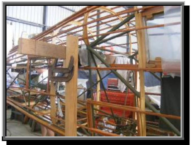
The wooden support, with clamps, in place. The ends of the fuselage have bars attached, which will help to spin the aircraft when the sleeve is finally attached.
