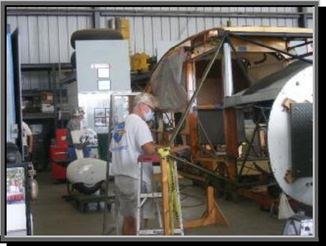
Here George is beginning to set a support for the fuselage prior to the sleeve fitting.
