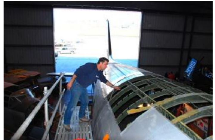
© Photo by Dan Newcomb Jeff Birdt working on removing the corroded "skin"
