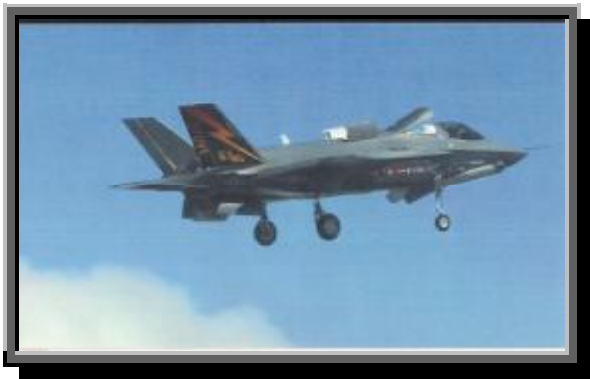
To the newest experimental Navy fighter, the Lockheed-Martin F-35 Lightning II , which can hover, land on a dime, and attain supersonic speeds.
