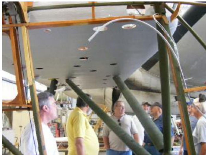
© Photo by Dave Flood The F-24R’s left wing has just been attached to the fuselage after it was covered and painted. The team members are basking in the afterglow of the event. Robert Albee is framed by the gear struts.
