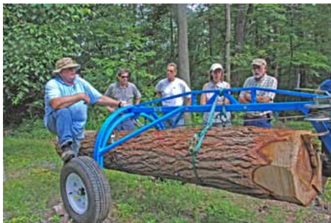
This log dolly can be used behind a tractor and can haul large logs out of the woods
